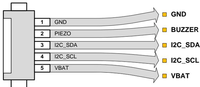
By default, the HERKULES III Powerboard is jumpered to supply PIN5 directly with the battery voltage.
