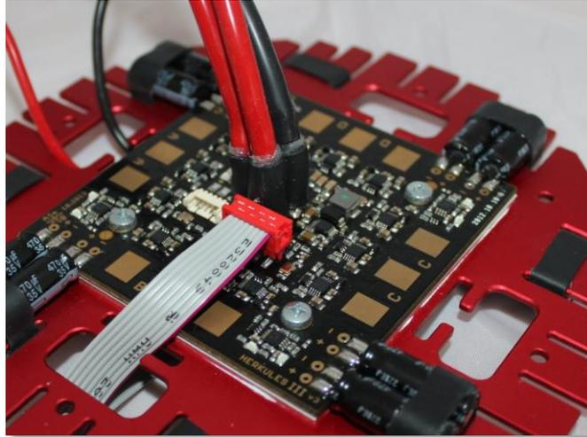
Remember to put the Telemetry Interface into the attached shrink-tube to protect it from short circuits and to secure fix the Molex connectors to the board.
