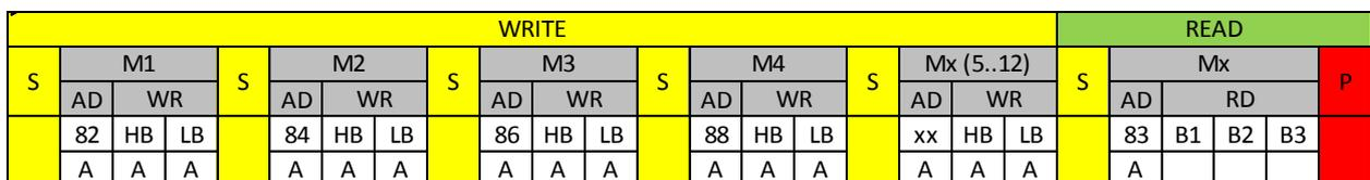
One frame should contain all setpoints for the motors (M1...16) but only one read parameter for one motor the diagnosis The address of the read parameter is increased after each communication frame and lowers therefore the update rate of the I2C communication interface.
