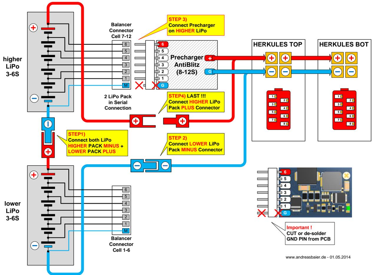
Figure 13 – Precharger Connection for 12S Batteries with double pin connectors
