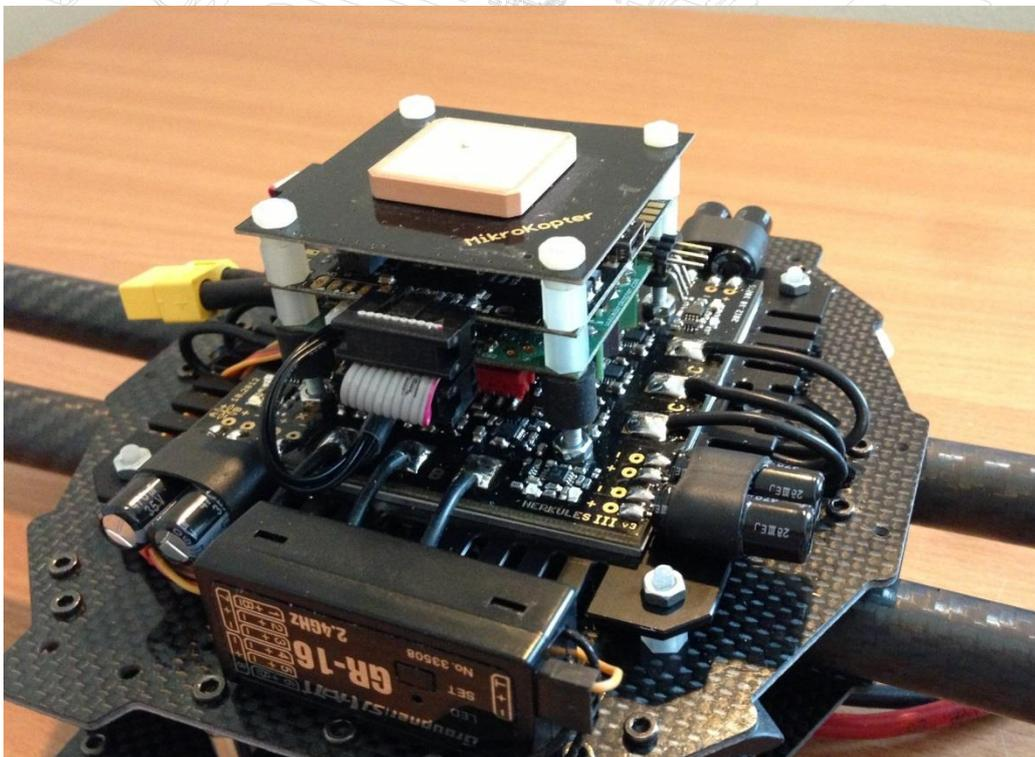
Figure 37 – Example Connection Scheme : HERKULES III with Mikrokopter FC2.1 ME
