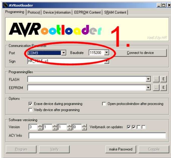
First select the correct Comport of the USB-to-HERKULES III - ProgTool. The Port must not be set to "AUTO". You have to set there the real Comport which is used by the ProgTool.
