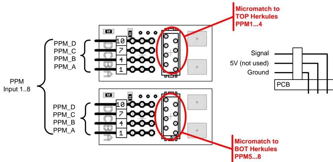
Figure 7 - PPM/I2C Breakout Board ready assembled
