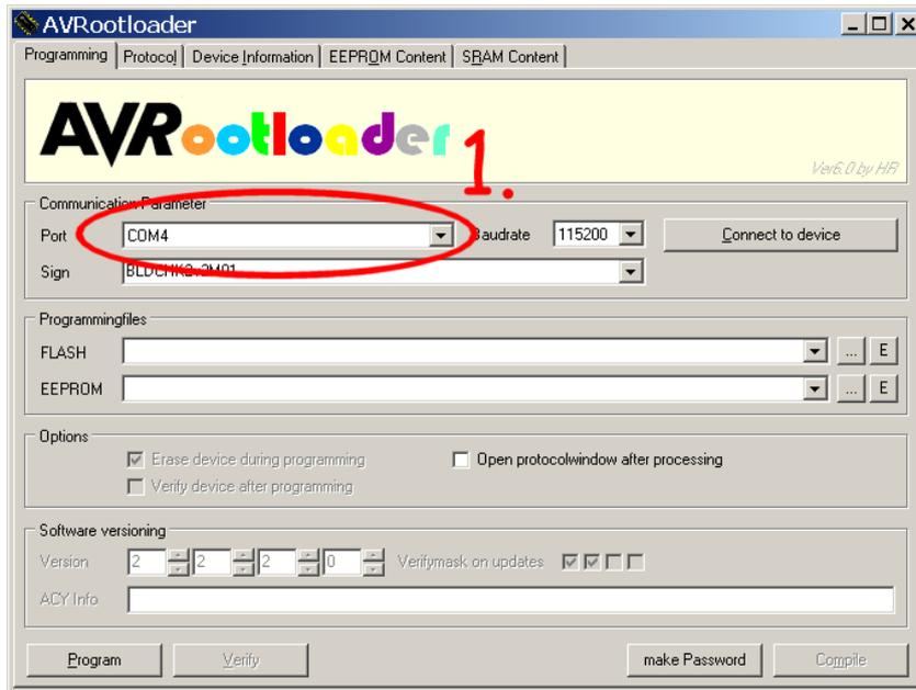
First select the correct Comport of the USB-to-HERKULES III - ProgTool. The Port must not be set to “AUTO”. You have to set there the real Comport which is used by the ProgTool.
