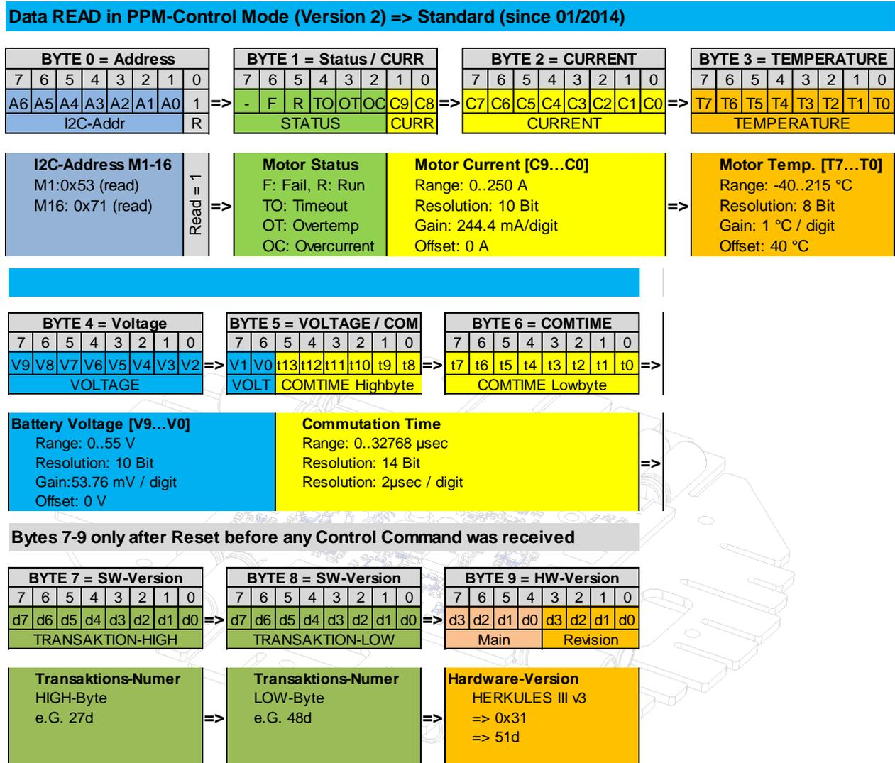
**BYTE0** is the read address with RW-Bit = 1. Same 7-bit address as write-mode but with RW-bit set different.
