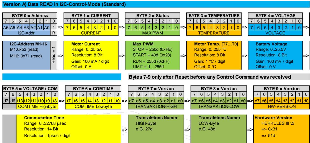
**BYTE0** is the read address with RW-Bit = 1. It's the same 7-bit address as in write-mode but with RW-bit set different.
