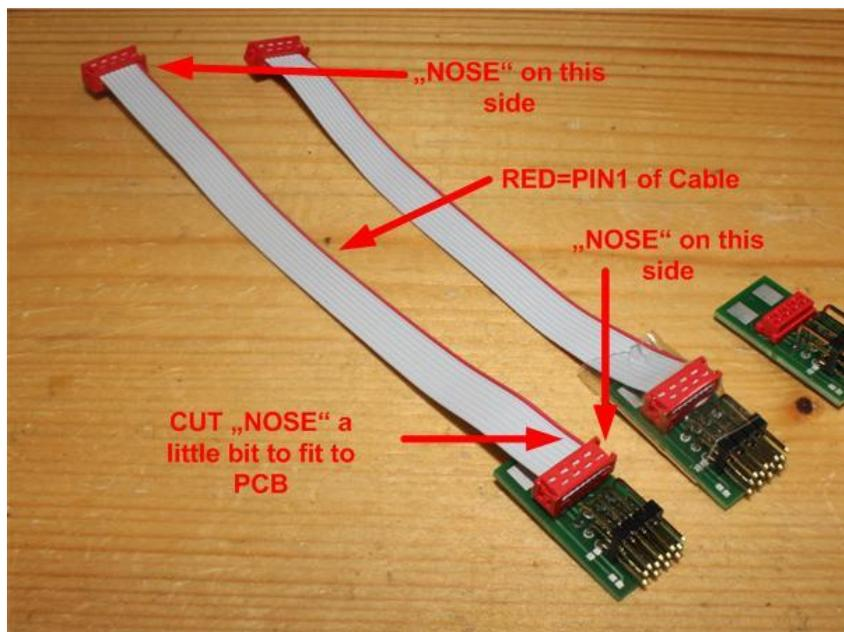
The connection between PPM breakout board and HERKULES III ESCs is done with a flat ribbon cable with pressed red Micromatch connectors. If the red connector does not fit correctly on the breakout board, cut the small "Nose" from the connector.
