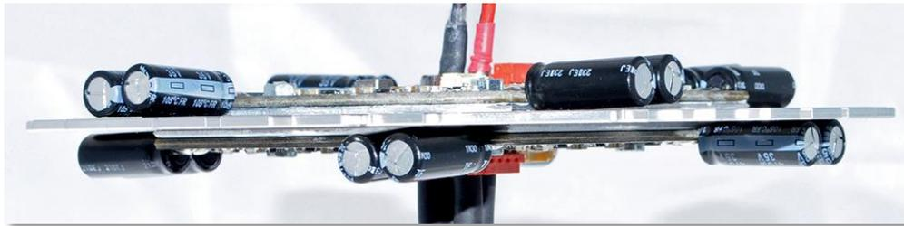
As the bottom HERKULES III is mounted “flipped” across the B-D axis (A-C exchanged) the motor addresses have to be set accordingly. The top board has the bootsigs written in superscript “**A,B,C,D**” and the bottom board has the bootsigs written in subscript “**e,f,g,h**” (which are linked on the physical “A,B,C,D” ESCs on the bottom board).
