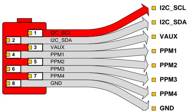
On Pin VAUX the HERKULES III Internal 8V/1.5A Supply Voltage is available. This can be used e.g. for the HERKULES III Telemetry Interface Board or supplying an External Flight Control.
