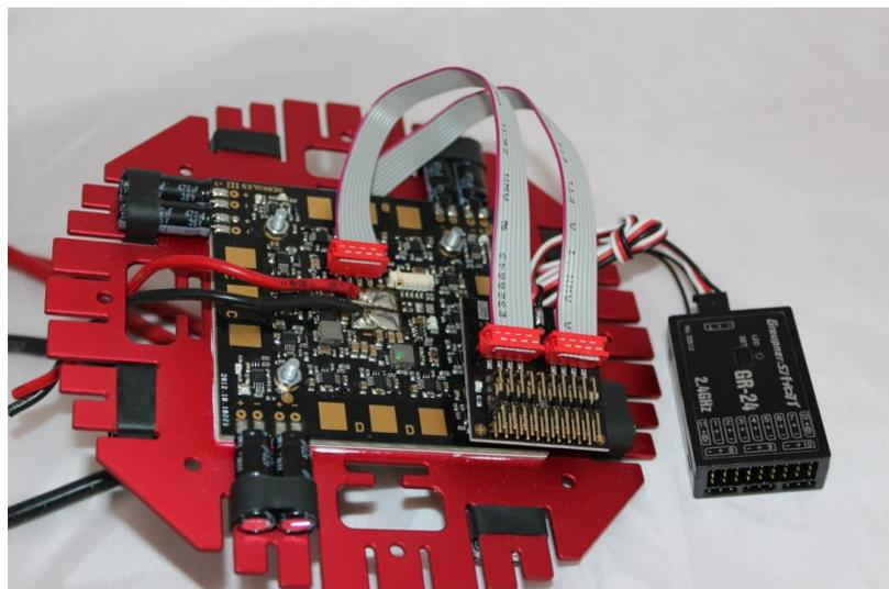
Figure 23 – Example Connection Scheme : HERKULES III with DJI-Wookong M
