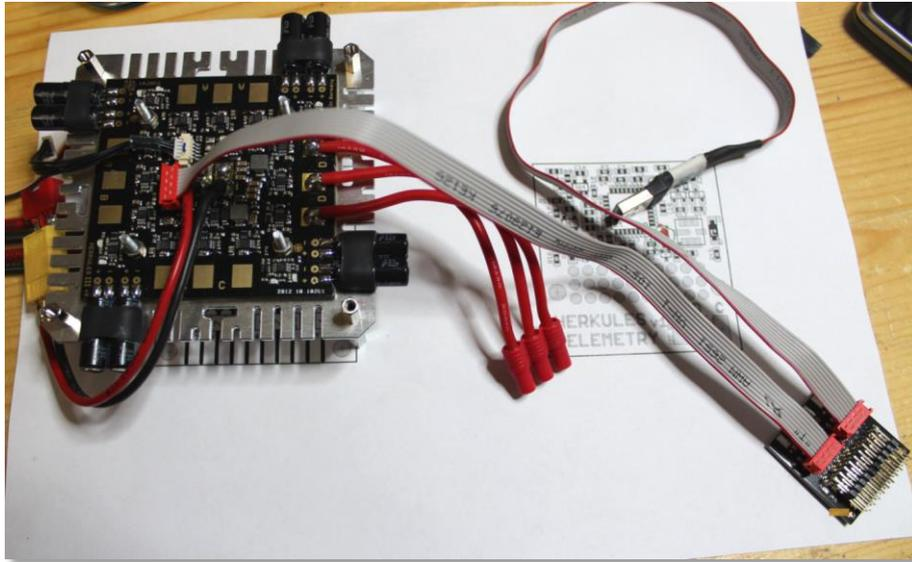
When the USB-to-HERKULES III ProgTool is connected to the Telemetry Interface, both HERKULES III Powerboard's can be accessed and programmed without direct connection of the programmer to the HERKULES Boards.
