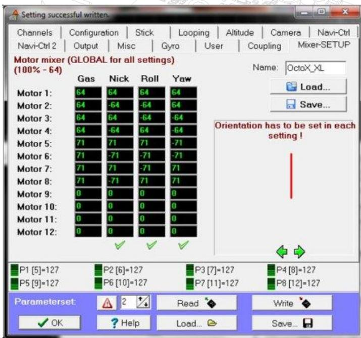
**Note:** In order to improve efficiency of the Coaxial-Setup, it is possible to reduce the motor setpoint values of the TOP Motors by 5-10%. This increases the overall efficiency and improves flight time.
