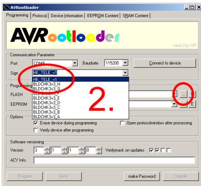
Select the one of the target ESC bootloaders in "Sign" which are ending with M01 to M04 or A to F.
