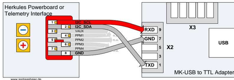
The programming adapter can be connected directly on the HERKULES III Powerboard or on any of the Telemetry Interface Micromatch connectors. Both Connectors on the Telemetry Interface are equally usable for programming the whole system. Remember: The supply of the Telemetry Interface boards is done from the HERKULES III Powerboard, therefore must be always one connection via flat ribbon cable to any of the HERKULES III Powerboard connected.
