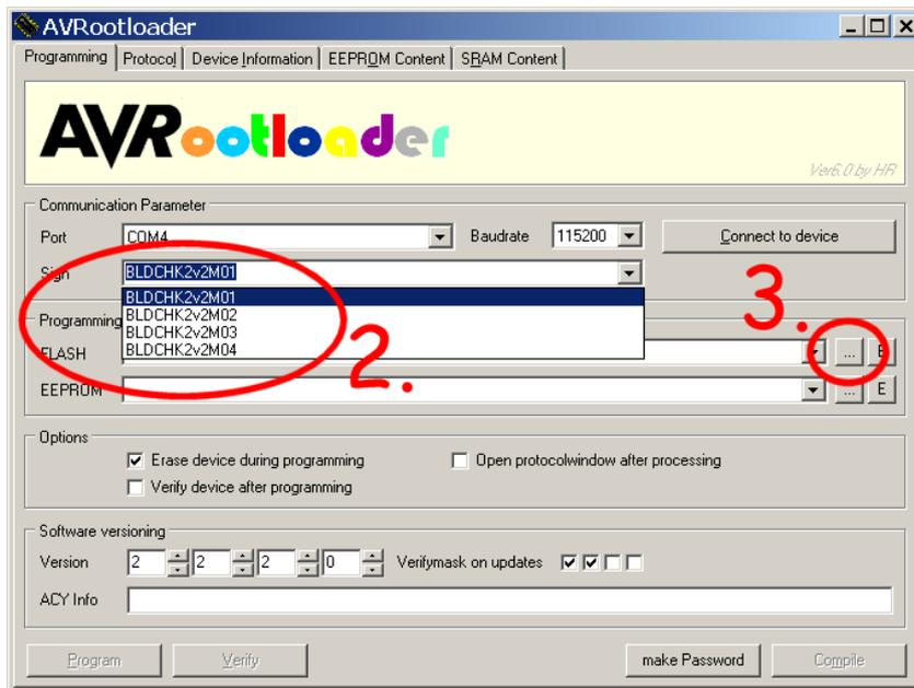
Select the one of the target ESC bootloaders in “Sign” which are ending with M01 to M04 or A to F.
