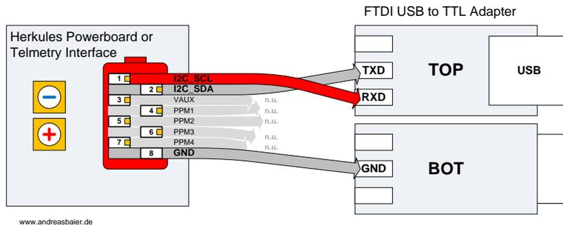
Figure 18 – HERKULES III Programming Tool with MK-USB Adapter
