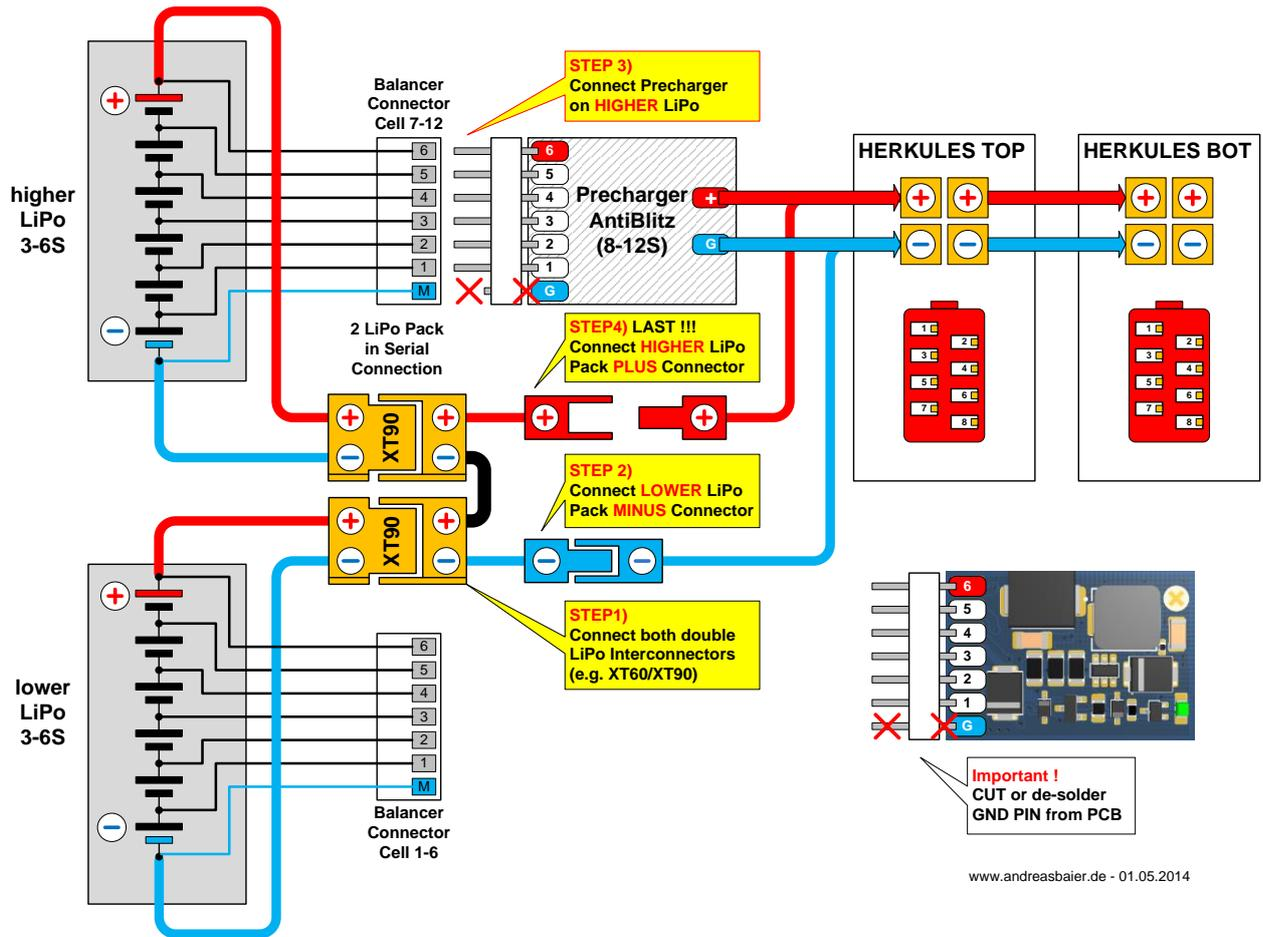
Figure 14 – Precharger Connection with 7s and double pin connector
