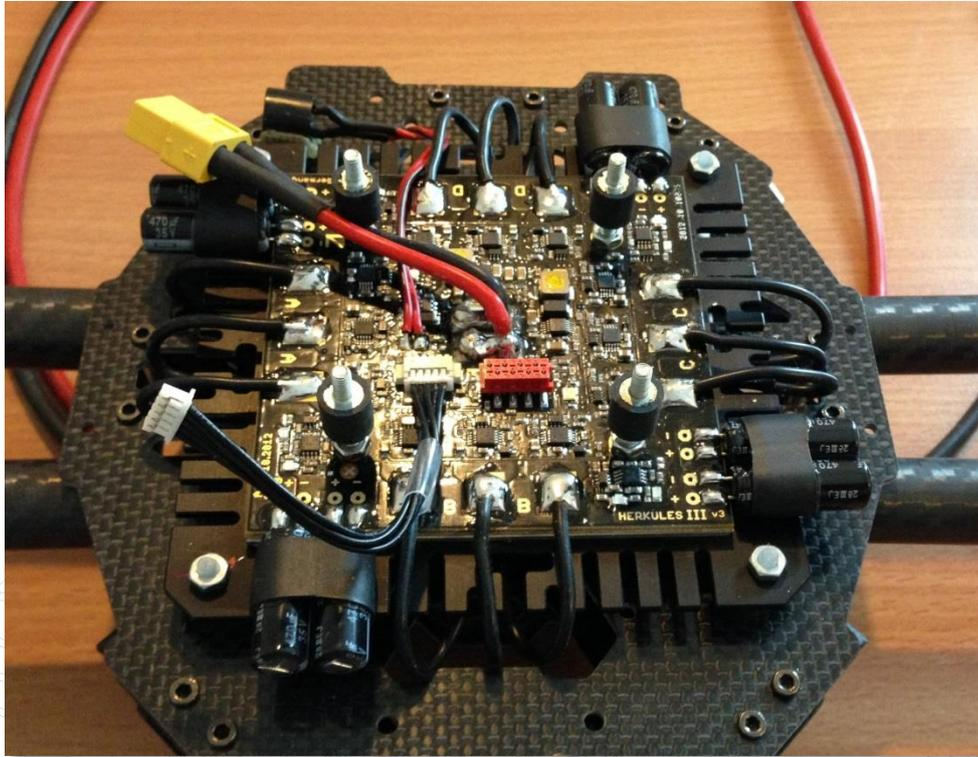
Figure 36 - Typical Setup with Mikrokopter Flight Control
