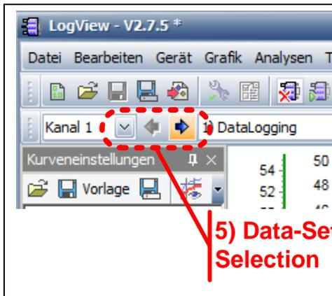
Click the small blue arrow on the channel selection bar to switch between one of the six Herkules III Data channels.
